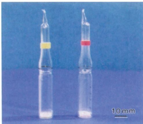
Figure 1. Vacuum-sealed ampoules with freeze-dried mouse spermatozoa. The white powder at the bottom of each ampoule is the dried CZB medium containing spermatozoa.
